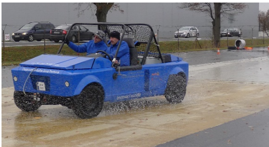
Fig. 1. Experimental vehicle on sliding surface
