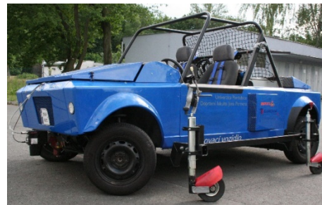
Fig. 2. Experimental vehicle with ASC
